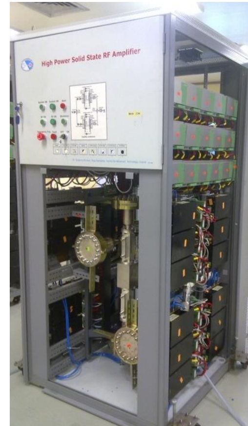
12.5 kW, 505.8 MHz Solid State Amplifier
