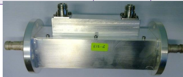
Designed 1 kW, 5 kW and 20 kW directional couplers
