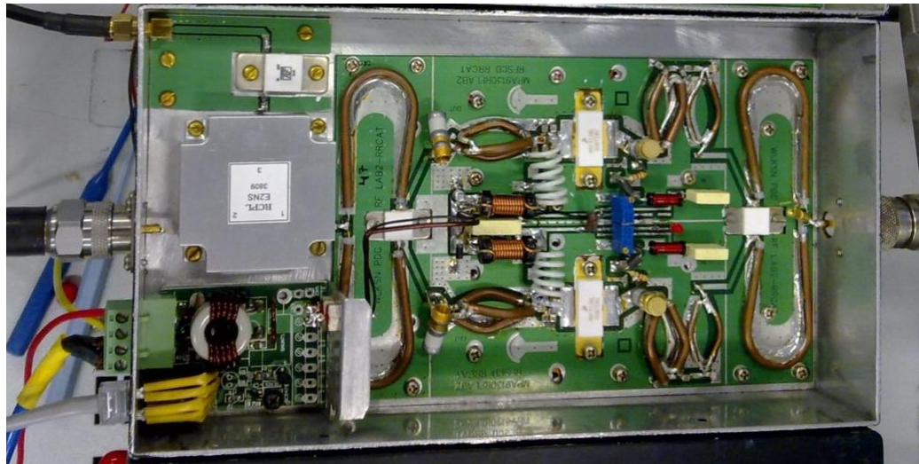
500 W solid state amplifier module
