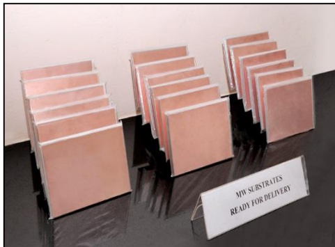
Substrate developed by C-MET ( \epsilon_r=4.3 , Loss factor=0.0018, \tau_{gr}= 30 \text{ ppm}/^\circ\text{C} ) 2010
