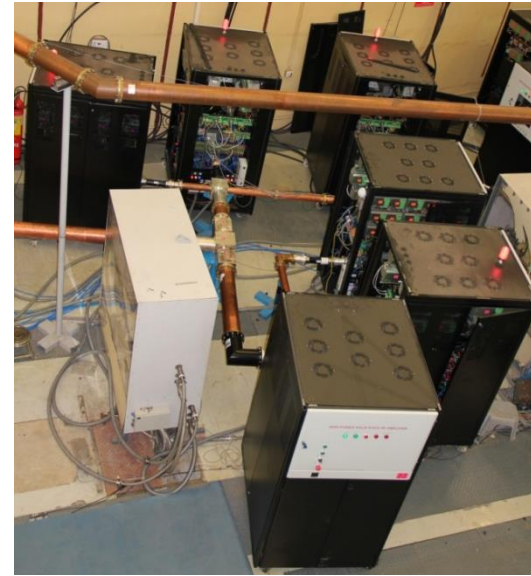
Fig 2: 75 kW SSPA coupled to RF cavity # 2
