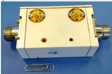
Designed 1 kW, 5 kW and 20 kW directional couplers
