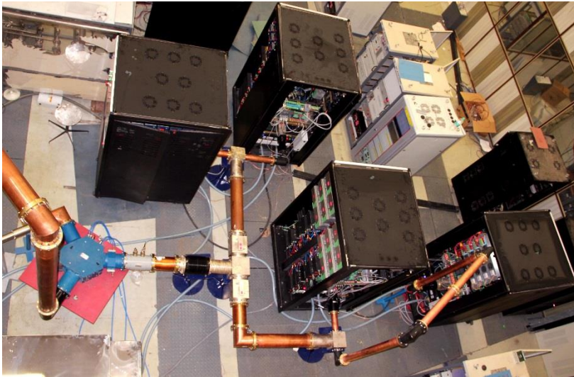
Fig 1: 50 kW SSPA coupled to RF cavity # 1
