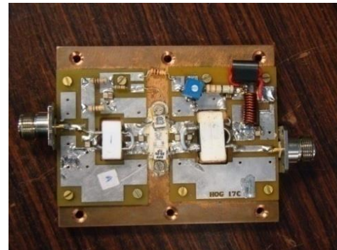
One of the four amplifier Modules (250 W ) used in 1kW amplifier
