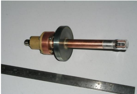
Sensing Loop Coupler for Indus-1 RF cavity @31.6MHz
